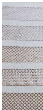
Figure 4. Five initial TPU samples of varying lattice structures developed by EOS Singapore Ptd Ltd and A-star
